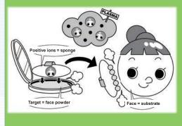
Positive ions impact a target so that atoms in the target are thrown up in the plasma. They are deposited on the substrate. This phenomena is so-called "sputtering".
