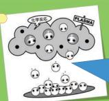
In plasma, electrons collide with hydrocarbon gas so that hydrogen and carbon are produced. Then, carbon atoms are deposited on the substrate.
