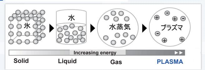
It is well-known that the matter changes with increasing energy, that is, solid (ice), liquid (water) and gas (water vapor). Furthermore the gas gets energy, the gas has negative and positive charged particles, it is so-called the fourth matter "PLASMA". The difference between the gas and the plasma is that the plasma is shining. In the nature world, there are thunder, aurora and sun. We can also see a fluorescent lamp and a flame.
