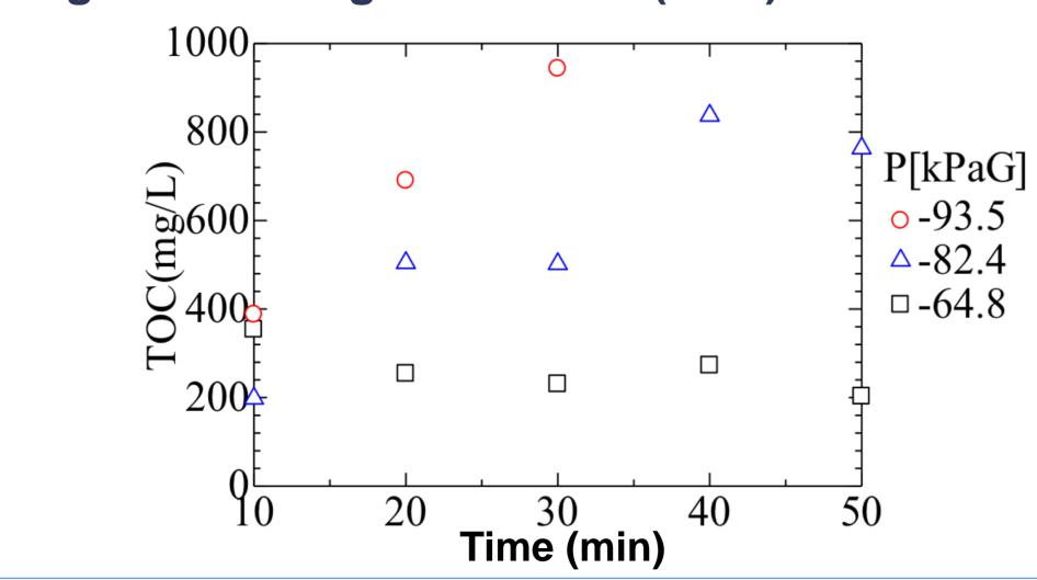
According to the increase in circulation time, TOC increased. Longer precessing time leads to progress of cell breakage.
